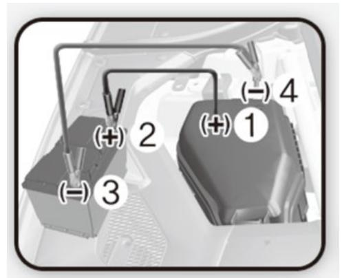
5. Start the vehicle with the booster battery, then start the vehicle with the discharged battery.
