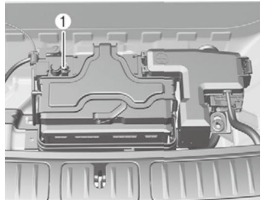
B. Disconnect the 12V auxiliary battery negative(-) terminal ①.
